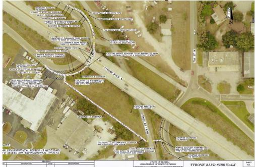
Frontage Road Sidewalks being connected by curve sidewalk + straight sidewalk across field, Pinellas Trail, over ditch, through guard rail to Tyrone Mall.
